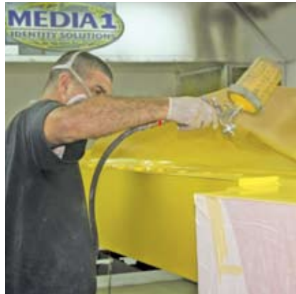
After having applied a red basecoat to the sign, Media 1’s paint team covered unmasked areas with four coats of yellow, satin-finish Matthews urethane paint.
