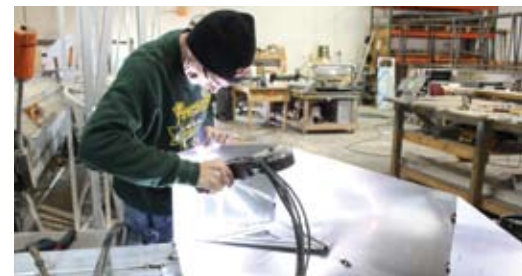
Next, fabricators shaped the aluminum sidewall and welded it around the sign's perimeter. Four, 4-in.-sq., aluminum legs served as a telescoping mounting system to slide the sign into the building-mounted framework.
