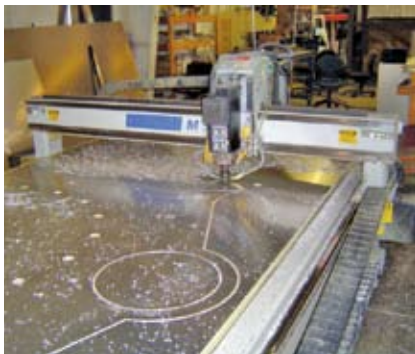
The shop's Multicam 3000 CNC router shaped the sign's aluminum skeleton from 0.125-in.-thick, 5052 aluminum.
