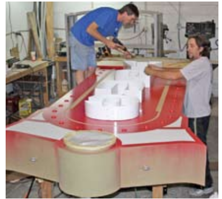
After having fabricated the letters using Arete’s channel-letter fabrication system, fabricators mounted the letters to the sign, wired them with double-stroke neon and covered them with clear, acrylic faces.
